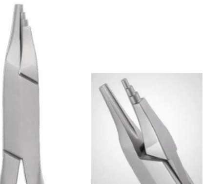
3000/98 Tweed – Short ø max 0,5 mm / .020" mm 135 Designed to form precise omega loops. Long grooved beak internally smoothed. Short type.
