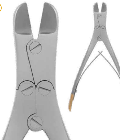
9952/160 TC ø max 1,5 mm / .060" mm 170 Double action system for heavy wires, reduce effort on cutting.
