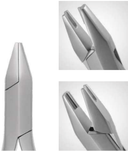
3000/171 V-Stop ø max 0,55 × 0,64 mm ø max .021" × .025" mm 130 For bending archwire in V-form, in order to avoid any movement.
